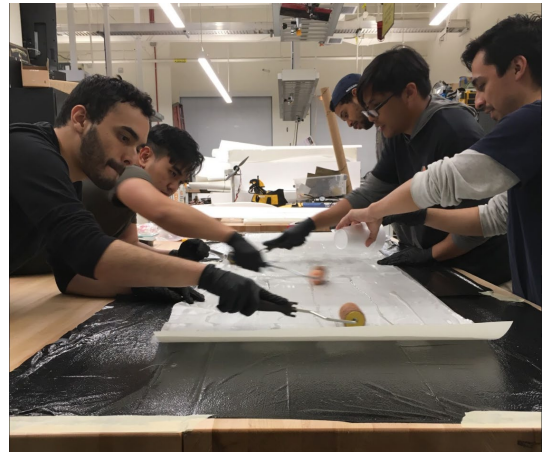
Figure 20: Members from the 2018-2019 SDSU DBF Team preparing a fiberglass layout for the 2019 competition plane’s wing.
